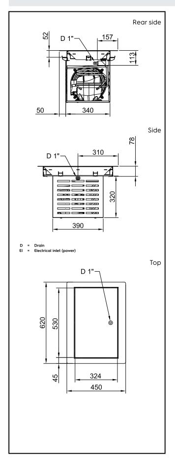
Drop-In Drop-in refrigerated quartz surface - IGN
